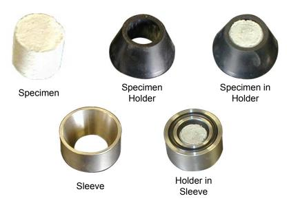
2. Place the sleeve between the pressure plates on the permeameter.
